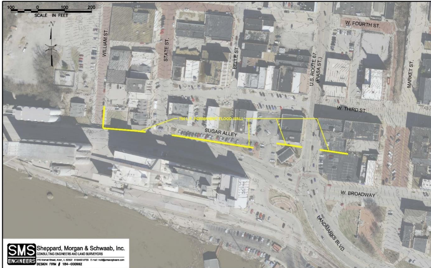
Figure 19. Structural Option 5: Alton, IL Proposed Floodwall Alignment
