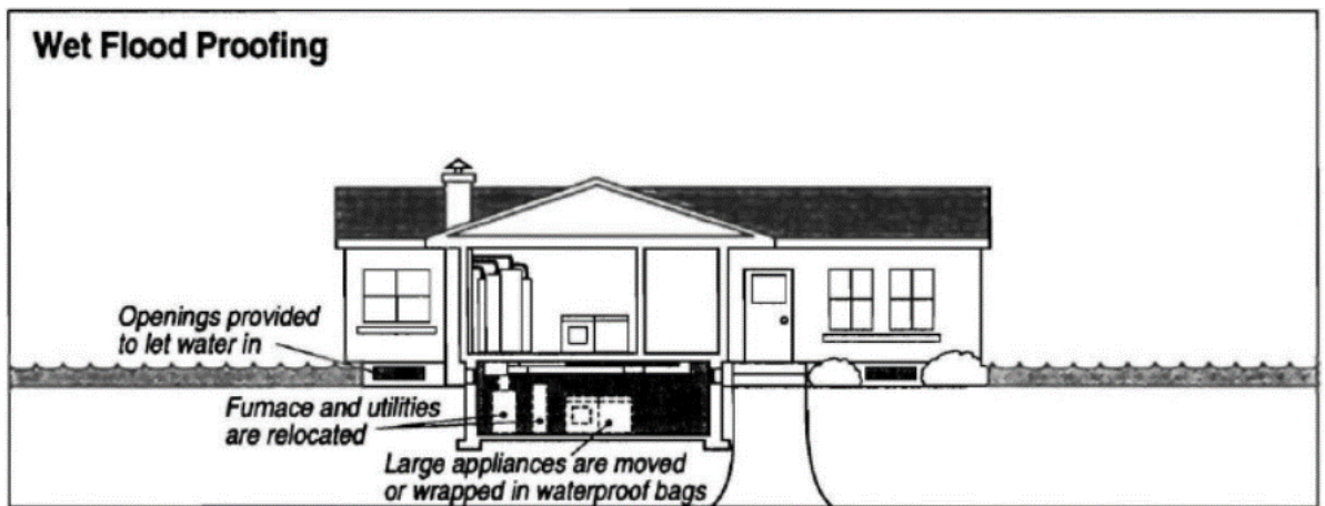
Figure 5. Wet Flood Proofing Diagram
